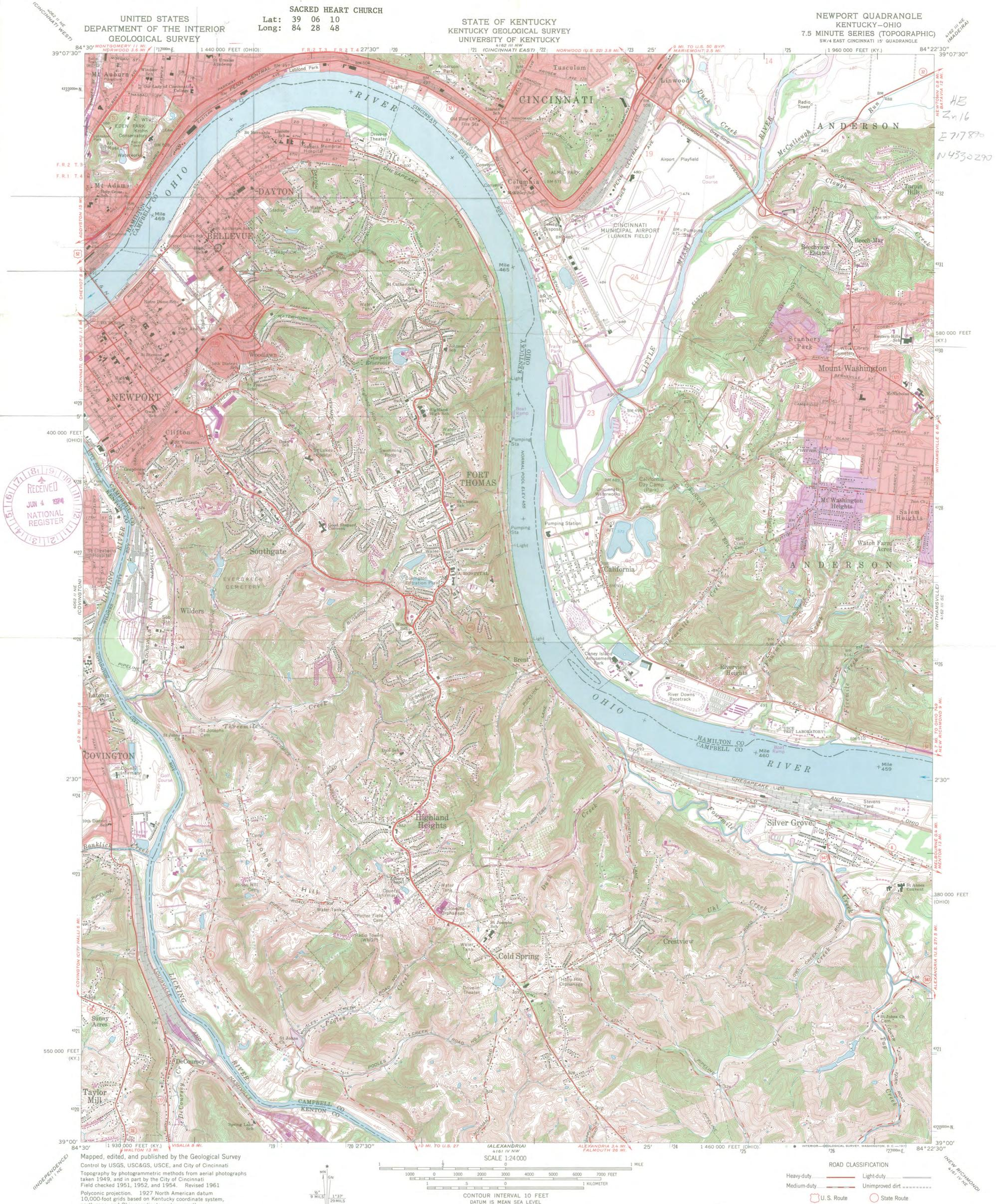
10,000-foot grids based on Kentucky coordinate system, north zone, and Ohio coordinate system, south zone 1000-meter Universal Transverse Mercator grid ticks, zone 16, shown in blue
