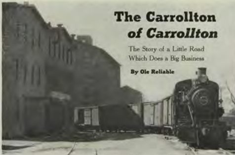
The Carrollton's spur leading into the Carrollton Furniture Manufacturing Company has such a sharp degree of curvature that the engine cannot negotiate it. The narrowers working is done by shoving a string of freight cars back into the plant to couple onto the cars to be hauled out. Engines are placed for leading in the same manner.
